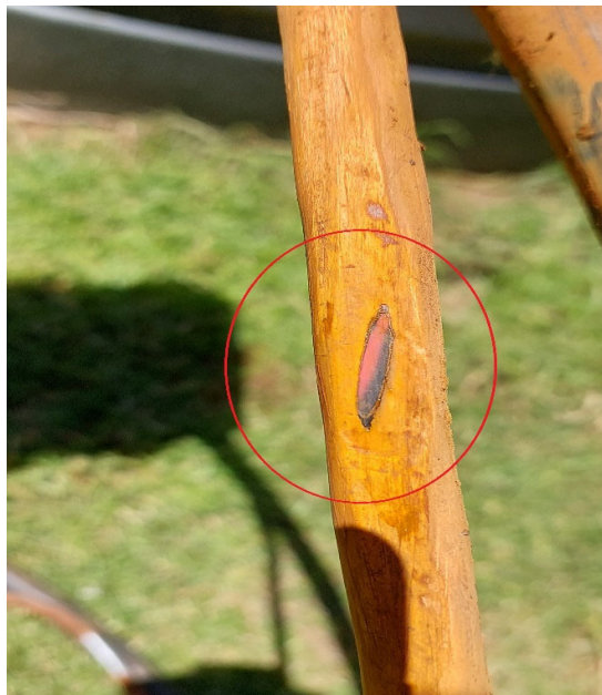
Damaged submersible pump electrical cable.
