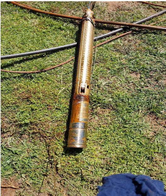
Condition of pumping equipment showing Iron Bacteria.
