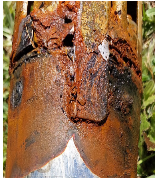
Condition of pumping equipment showing Iron Bacteria.
