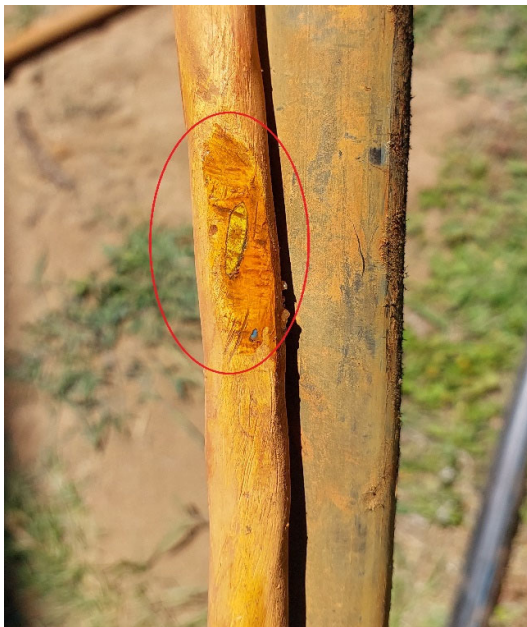
Damaged submersible pump electrical cable.
